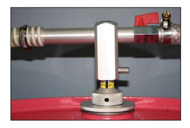
The required concentration can easily be obtained by setting the regulator to the correct number.
