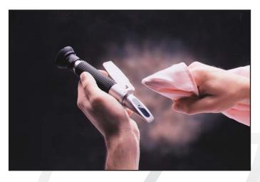
The only maintenance required is cleaning with a dry cloth after use
