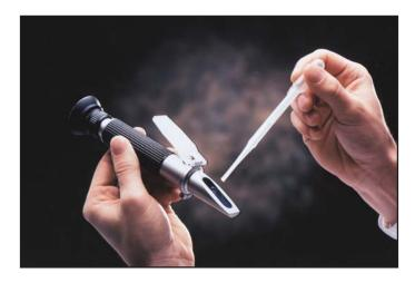
Place a few drops of metalworking fluid on the Refractometer prism with the plastic pipette supplied with the instrument
