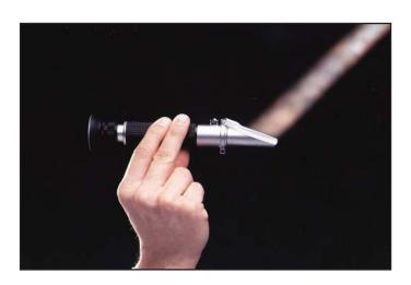
Point the Refractometer at a strong light source and adjust the scale focus and scale calibrate knob gives a reading on the Refractometer scale
