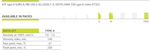
Universal monograde oil designed for torque converters in heavy mining, construction and other machinery, requiring oil performance level complying with Allison C4 and
