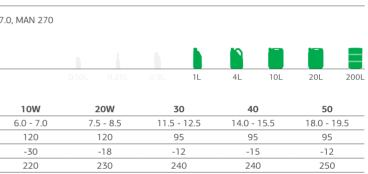
Special oil for lubrication of railroad locomotive diesel engines, manufactured by General Motors, Electrical Division and other railroad manufacturers, with or without turbocharging. This is a zinc-free type of oil, designed for lubrication of engines with silver-alloy made piston pin bearings. Provides effective protection against wear and
