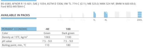
PERMANT ECONOMIC 100 is intended for central heating system protection against: freezing, rust, corrosion, cavitation and foaming, thus providing maximum cooling
