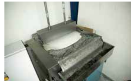
Hydrostatic band filter for filtering particles and metal chips from the coolant.
